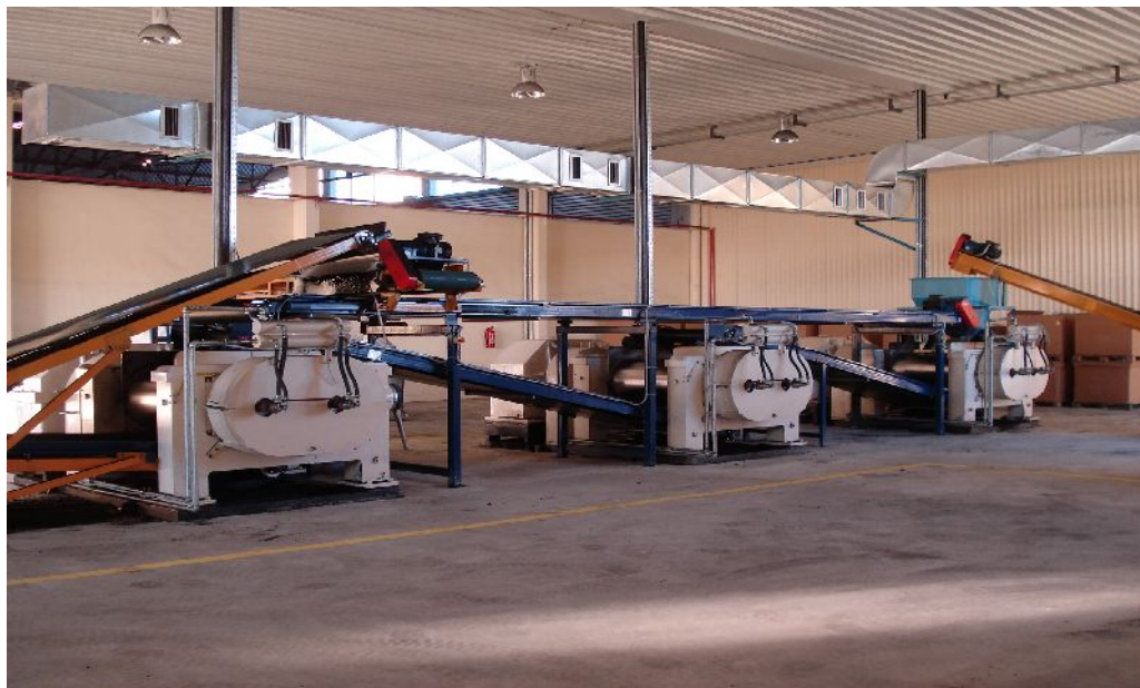
Fig.1: Illustration of the three de-vulcanizing roller – mills with all the necessary auxiliaries, roller mill cooling system etc.
